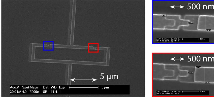
Figure 2.12: SEM image of a dc-SQUID. The red and blue rectangles show the positions of the Josephson junctions. Image taken from the supervised thesis [48]
