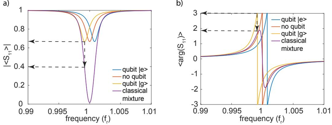
Figure 3.4: Calculated signal reflected from a coupled qubit-resonator system. Average amplitude (a) and phase (b) for different qubit states in dependence of applied frequency in units of the resonators bare resonance frequency  $f_r$ . Average amplitude and phase are the actually measured quantities in the experiment.
