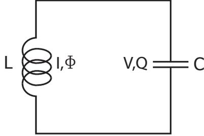
Figure 1.6: Parallel connected LC-oscillator
