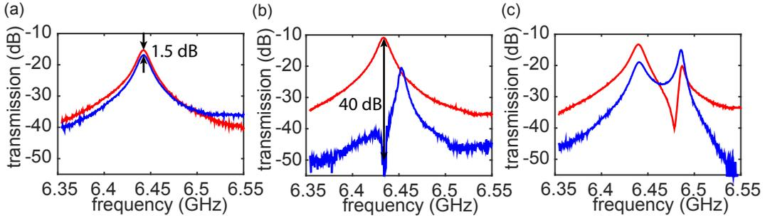
Figure 5.4: Through- (red) and cross-measurements (blue), obtained for three different flux values. (a)  $\Phi_{\text{ext}} = \Phi_0/2, |g| \gg |\Delta|$ : strongly coupled regime, only the mode  $\Omega_1$  is shown. (b)  $\Phi_{\text{ext}} = 0.468\Phi_0/2, |g| \simeq 0$ : decoupling point. (c)  $\Phi_{\text{ext}} = 0.439\Phi_0/2, |g| \simeq \Delta$ .
