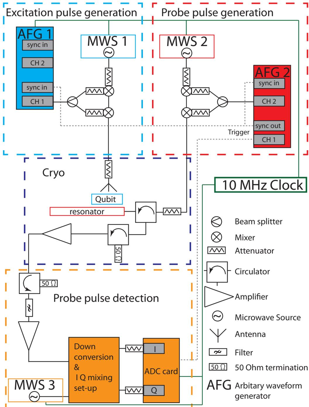
Figure 3.5: The time domain set up consists of the sample in the cryostat (dark blue dashed box), the qubit excitation pulse generation (light blue dashed box), the resonator probe signal generation (red dashed box) and reflected probe signal detection (orange dashed box). All devices are synchronized by a 10 MHz-clock and events are triggered by the channel 1 of the AFG 2 (gray dashed box).
