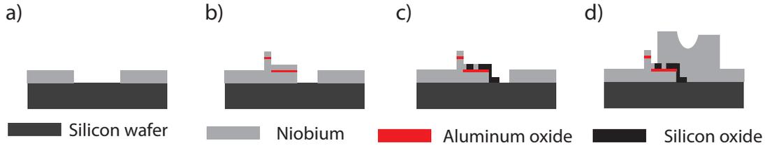
Figure 2.8: Fabrication process for Nb-junctions. (a) Wiring layer is deposited. (b) The Nb/AlO<sub>x</sub>/Nb trilayer is placed in a lift-off process. (c) The junction is defined in an etching process and an SiO<sub>x</sub> insulation is applied. (d) A top electrode is attached to connect the top layer of the junction with the wiring.
