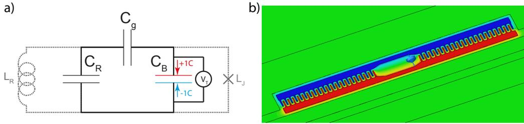
Figure 2.16: Simulation of the transmon capacitance. (a) Effective circuit and (b) the simulated structure. Here capacitance of the Josephson junctions is here taken into account as a lumped element. Charges of  $Q = \pm 1C$  are placed on the interdigitals electrodes of the transmon. The calculated potential is illustrated in the displayed color (red: high voltage, blue: low voltage).
