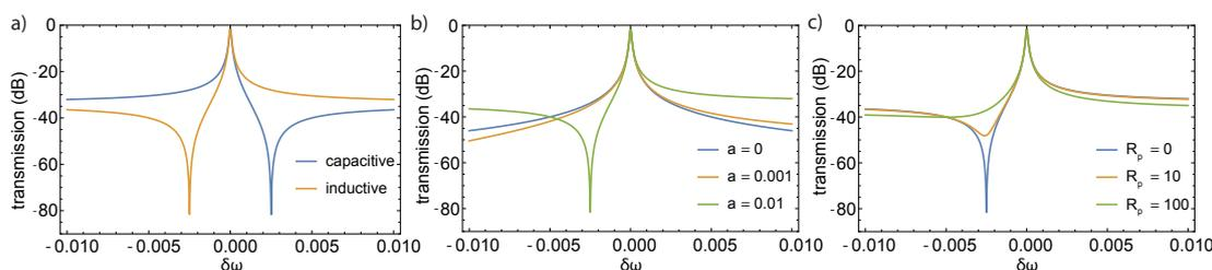
Figure 2.7: Fraction of transmitted power in logarithmic units as a function of the normalized excitation frequency  $\delta\omega = (\omega - \omega_r)/\omega_r$ .  $Q_{\text{ext}} = 10000$ ,  $Q_{\text{int}} = 50000$  are fixed in all subfigures. (a) The two types of coupling for  $b = -a$ . (b) Plots for different values of the parameter  $a$  with  $R_p = 0$ , (c) Effect of different  $R_p$  with  $a = 0.01$
