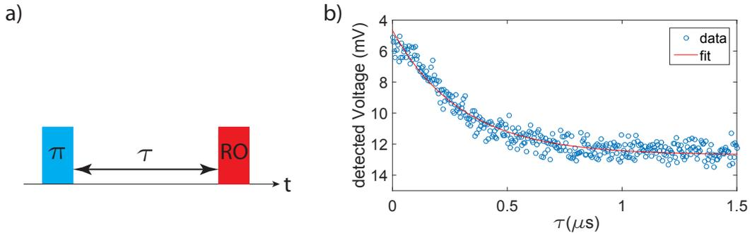
Figure 4.9: Measurement of the  $T_1$ -time. a) First, the qubit is excited by a  $\pi$ -pulse (blue). After a waiting time of  $\tau$  the qubit population is measured via a short probe pulse (red). b) Exponential decay of the qubit measured via the resonator response (blue dots). Fitting the data (red line) leads to  $T_1 = 298$  ns
