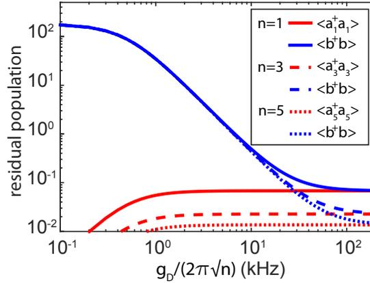
Figure 6.3: Number of excitations in the fundamental mode of the nanobeam (blue lines) and harmonics of microwave resonator (red lines) during sideband cooling using different resonator modes ( $n$ ). The color code is as follows: fundamental mode - solid line ( $n = 1$ ), 2nd harmonic - dashed line ( $n = 3$ ), and 4th harmonic - dotted line ( $n = 5$ ). Note, that we have assumed a fixed quality factor of  $Q = 10^5$  for all microwave modes in our calculations.
