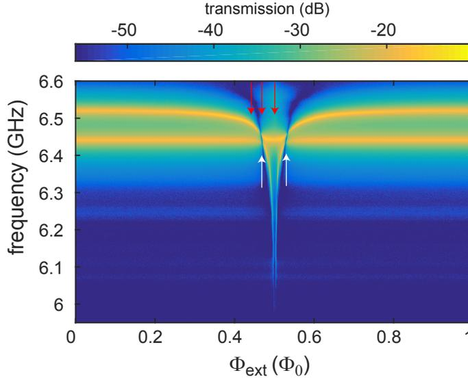
Figure 5.3: Cross-transmission from resonator A to resonator B as a function of the applied flux. Near  $\Phi_{\text{ext}} = 0.468 \Phi_0$  and  $\Phi_{\text{ext}} = 0.532 \Phi_0$  (white arrows), the resonators decouple and signal transmission is blocked. The red arrows mark the flux values, for which transmission vs. frequency cuts are shown in Fig. 5.4.
