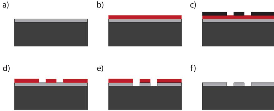
Figure 2.1: Fabrication scheme for niobium resonators. (a) Deposition of niobium on a oxidized silicon substrate by dc magnetron sputtering. (b) The substrate is covered with a  $1\ \mu\text{m}$  layer of resist. (c) Exposure with UV-light through an optical mask. (d) Development of the pattern. (e) Removing of uncovered niobium in a RIE system. (f) Finished structure after a chemical cleaning.
