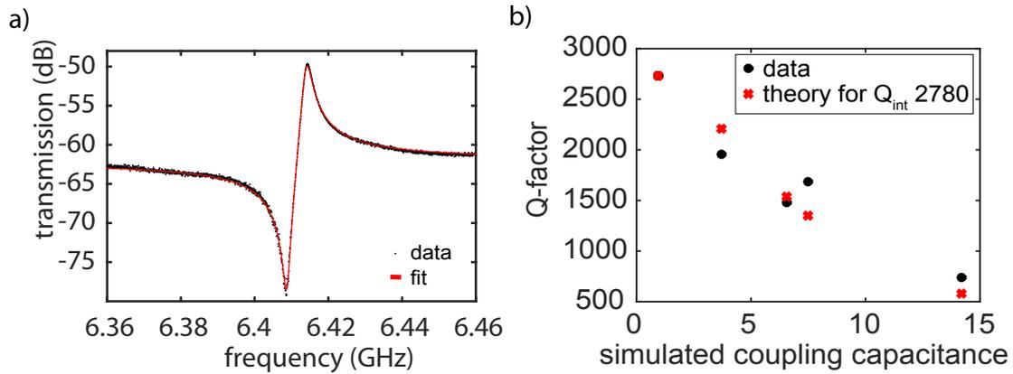
Figure 2.5: (a) Transmission spectroscopy of a undercoupled CPS resonator with an asymmetric lineshape. Black: data, red: fit to Eq. 2.1 parasitic path parameters parameters  $a = 0.13$  and  $R_p = 56 \Omega$  (b) Q-factor of different CPS resonators vs. simulated coupling capacitance. The black dots are measurement data, whereas the red crosses are simulations for  $Q_{\text{int}} = 2730$ . The data was acquired at 4.2 K
