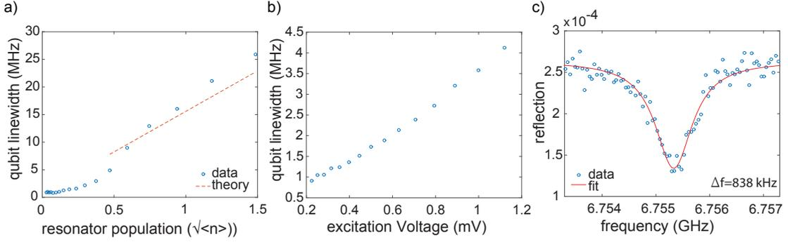
Figure 4.7: Qubit linewidth as a function of probe amplitude (a) and as a function of excitation amplitude (b). (c) shows the qubit transition with the best measured linewidth of  $\Delta f = 838 \text{ kHz}$ .
