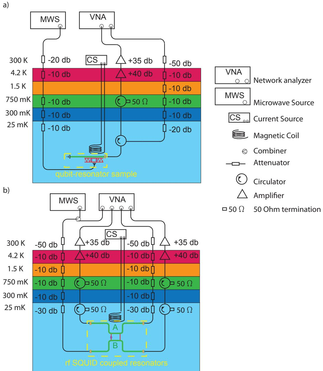
Figure 3.3: a) Set up for transmon qubit coupled to a resonator measurement. Sample yellow dashed highlighted. b) Set up for measurement of rf SQUID coupled resonators. Sample yellow dashed highlighted.
