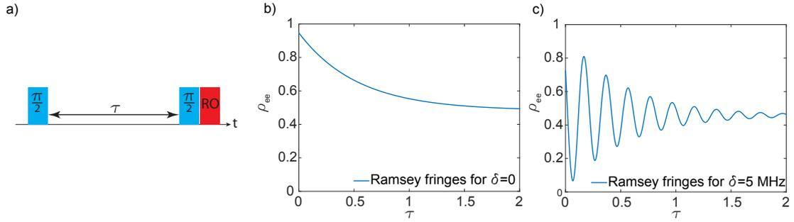
Figure 1.16: (a) Ramsey sequence consisting of two  $\pi/2$  pulses followed by a read out. (b) Excitation population for ( $\delta = \omega_q - \omega_d = 0$ ) depending on the waiting step  $\tau$ . (c) Same as (b), but for  $\delta = 5$  MHz
