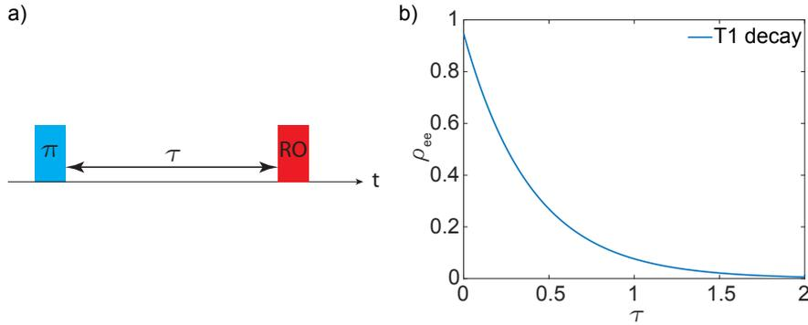
Figure 1.15: (a) Measurement scheme for  $T_1$  measurement. First the qubit is excited (blue) and after a time  $\tau$  the qubit state is read out (red). (b) The population decay leads to an exponential decay with characteristic time  $T_1$
