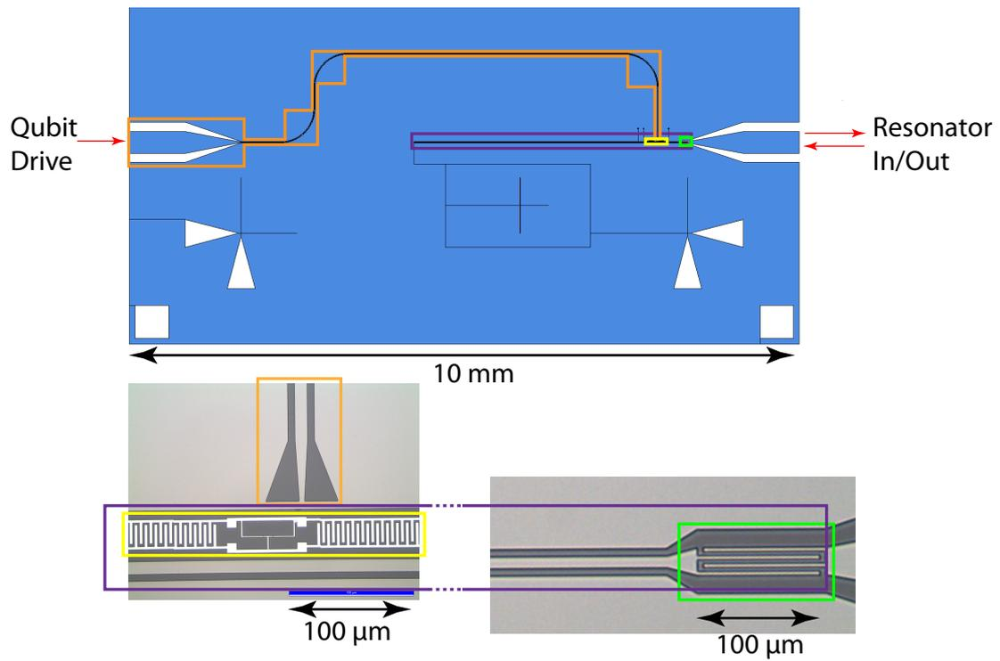
Figure 4.1: Technical drawing of the investigated circuit with photograph insets. The circuit consists of a  $\lambda/4$  resonator (highlighted in purple), which is connected to a read out port via a coupling capacitor (green). The transmon qubit (yellow) is capacitively coupled to the resonator at the voltage anti-node of the fundamental mode. The transmon qubit has an antenna (orange) for driving.
