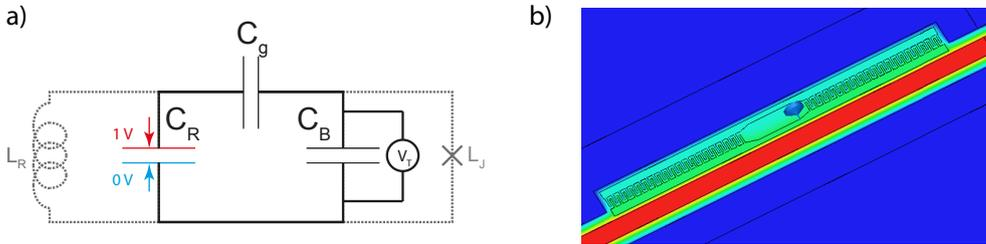
Figure 2.17: The simulation of the gate capacitance is shown here in (a) as an effective circuit and in (b) for a simulated structure. Here, a voltage of  $V_R = 1\text{ V}$  is applied to the resonator. The calculated potential is illustrated in the displayed color (red: high voltage, blue: low voltage).
