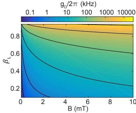
Figure 6.2: Envelope of Eq. (6.16) visualizing the achievable coupling rate  $g_D/2\pi$  in dependence of the SQUID's  $\beta_L$  value and the magnetic induction  $B$  for  $\Phi_{\text{rf}} = 0.01\Phi_0$
