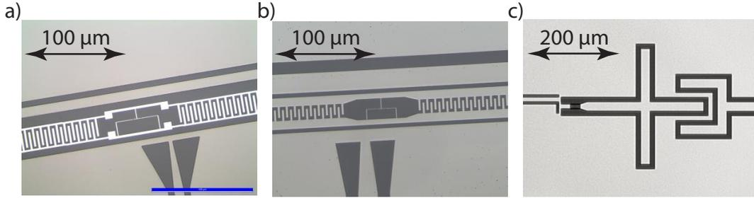
Figure 2.18: Different transmon qubits, which were investigated in this thesis. a) Transmon qubit, which data is presented in Sec. 4. b) Transmon qubit, which simulations are shown in Fig. 2.16 and Fig. 2.17. c) Transmon qubit with capacitor in CRW design.
