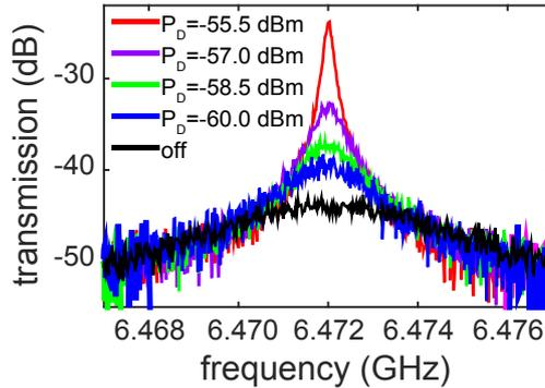
Figure 5.5: Through-transmission vs. frequency around the coupled mode frequency  $\Omega_1$  for  $\Phi_{\text{ext}} = 0.450\Phi_0$  and an additional applied flux-drive tone with frequency  $\omega_D/2\pi = 12.944$  GHz for different drive powers  $P_D$ . The drive power refers to the power at sample input.
