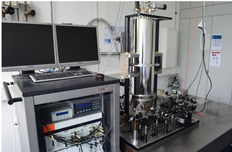
Figure 3.1: Overview of the lab. The cryogen level monitor, temperature controller and SPM controller are shown housed on the left rack while the optical table with the cryostat and the optical components for Raman spectroscopy are on the right [26].
