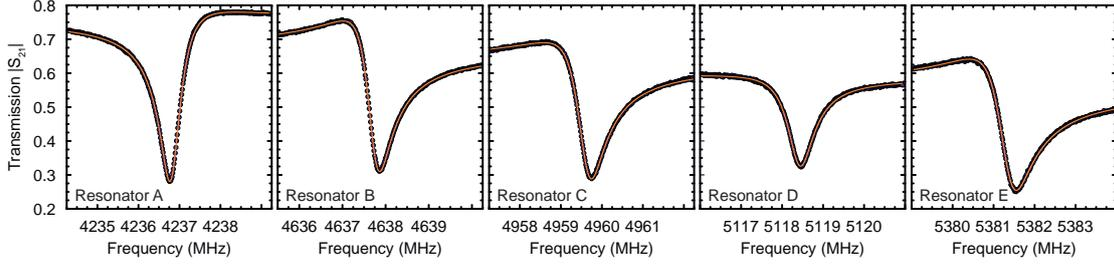
**Figure 3.4:** Calibrated microwave transmission  $|S_{21}|$  (symbols) as a function of the VNA frequency and at liquid helium temperatures, for the LERs A to E. The asymmetric lorentzian lineshapes are fitted using Eq. (3.6) (solid orange lines).
