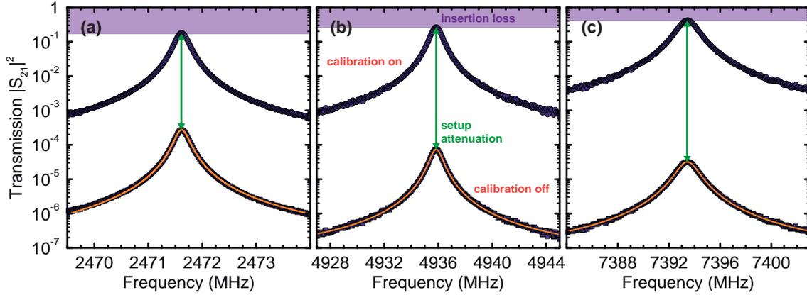
**Figure 3.1:** Power transmission of the CPWR at liquid helium temperatures as a function of the VNA frequency, for the fundamental (a), first (b) and second (c) harmonic resonator mode. The squared symbols show the transmission of the cryostats microwave cabling and the CPWR, fitted using a Lorentzian function (solid orange line). The round symbols show only the transmission through the CPWR, with the microwave cabling attenuation calibrated out.
