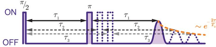
**Figure 4.11:** Schematic spin-echo pulse sequence. Repeatedly applying the sequence, while increasing the evolution time  $\tau$ , results in a decreasing echo signal. The characteristic time constant of the decreasing echo signal corresponds to the coherence time  $T_2$ .
