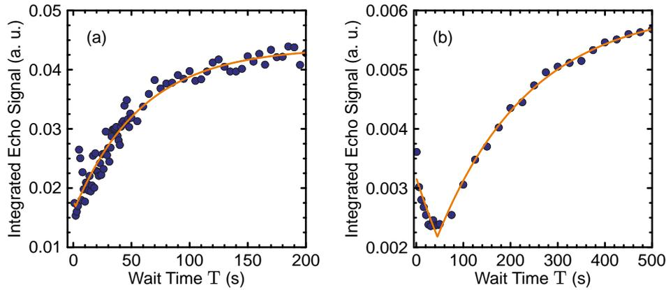
**Figure 4.21:** Integrated echo signal as a function of the wait time  $T$  obtained from an inversion recovery spectroscopy on the hybrid system at 50 mK, using the CPWR and LER (symbols in (a) and (b), respectively). The solid lines represent a fit to the echo signal, with the proportionality given in Eq. (4.11).
