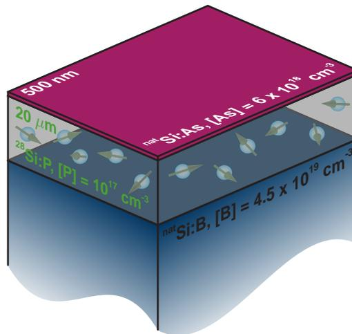
**Figure 2.8:** Schematic of the layer structure of the investigated phosphorus doped silicon. Originally the  $^{28}\text{Si}$  crystal was chemical vapor deposition grown on a heavily boron doped  $^{\text{nat}}\text{Si}$  substrate and cap by an arsenic doped  $^{\text{nat}}\text{Si}$  layer. To avoid any unwanted influences on the used microwave resonator the arsenic and boron doped layers were removed.
