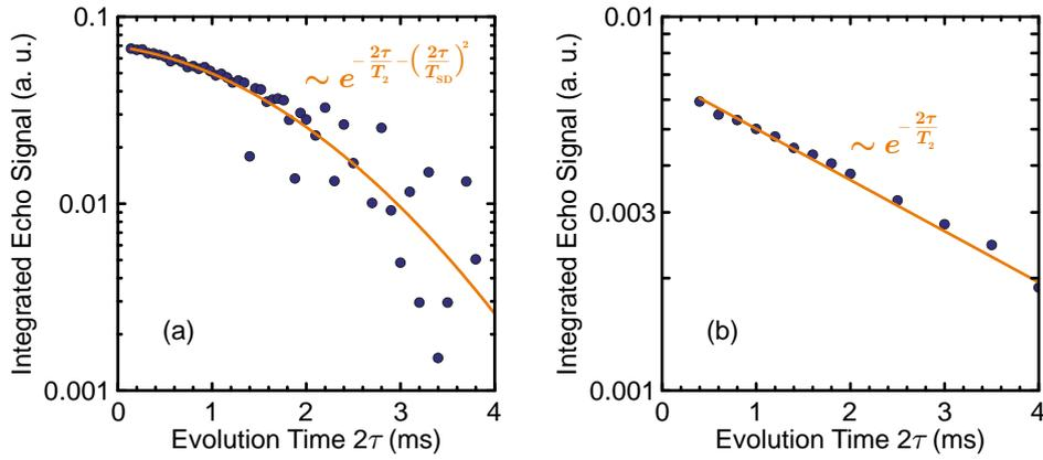
**Figure 4.15:** Logarithmic scaled integrated echo signal as a function of twice the evolution time  $\tau$  obtained from a Hahn echo spectroscopy on the hybrid system at 50 mK, using the CPWR and LER (symbols in (a) and (b), respectively). The solid lines represent a fit to the decaying echo signal, with the proportionality given in plot.
