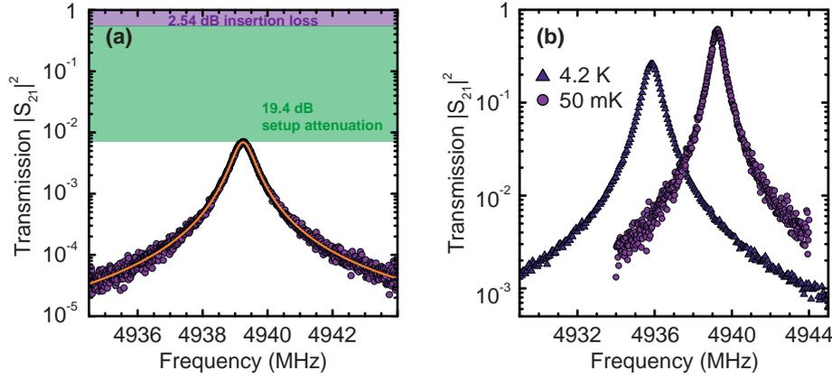
**Figure 3.3:** (a) Uncalibrated power transmission  $|S_{21}|^2$  (symbols) as a function of frequency of the CPWR's first harmonic mode at a temperature of 50 mK. The orange solid line is a lorentzian fit to the spectrum. The insertion loss of the resonator and the attenuation of the cryogen free dilution refrigerator microwave circuitry are accentuated by colored boxes. (b) Comparison of the calibrated transmission spectra measured at 4 K and 50 mK.
