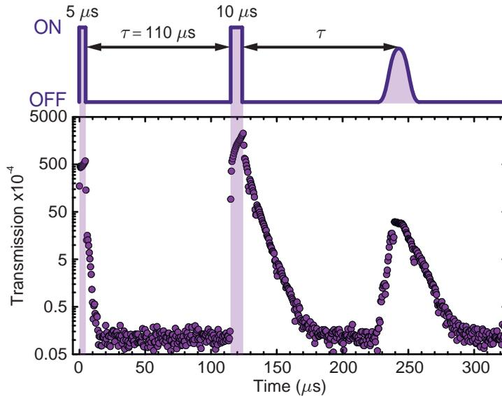
**Figure 4.14:** CPWR microwave transmission  $I^2/I_{\text{input}}^2$  as a function of the sequence time, for a temperature of 50 mK and  $I_{\text{input}}^2 = 2 \text{ nW}$ . The measurement trace is additionally illustrated by a schematic of the applied pulse sequence, highlighting the microwave pulses.
