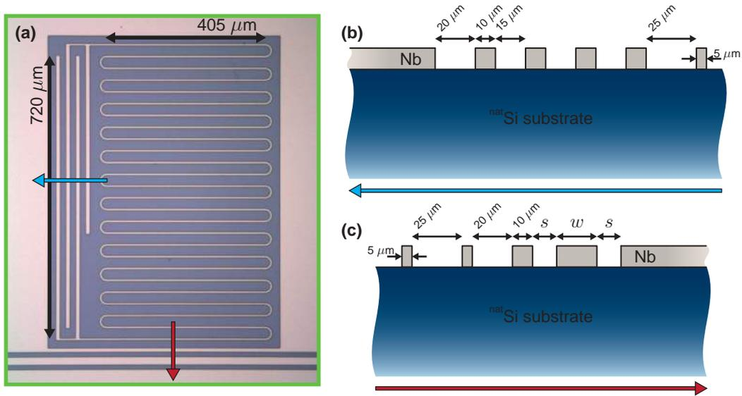
**Figure 2.3:** (a) Micrograph image of a niobium lumped element resonator. Additionally part of the adjacent CPW transmission line can be seen at the bottom of the image. (b) Schematic cross-section of the finger capacitor structure of the LER, where the blue arrow in (a) shows the location of the cross-section. (c) Schematic cross-section of the inductor and the alongside running CPW, where the position of the cross-section is indicated by the red arrow in (a).
