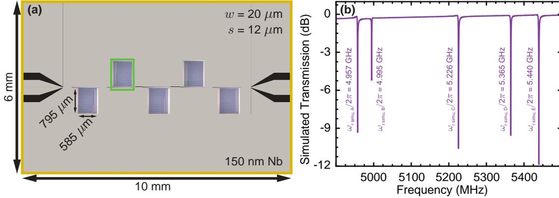
**Figure 2.4:** (a) Image of a niobium lumped element resonator chip with five resonators coupled to a common CPW transmission line. The LERs are micrograph images, while the rest of the chip is illustrated schematically. The resonator shown in Fig. 2.3 (a) is marked with a green box. (b) CST microwave studio simulation of the microwave transmission of a similar resonator chip shown in (a).
