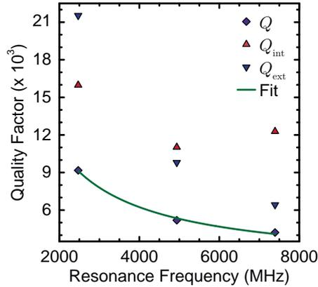
**Figure 3.2:** Loaded, internal and external quality factors of the CPWR at liquid helium temperatures as a function of the harmonic mode number. The resonance frequency dependence of the loaded Q-factor is described by Eq. 3.4 (solid green line).
