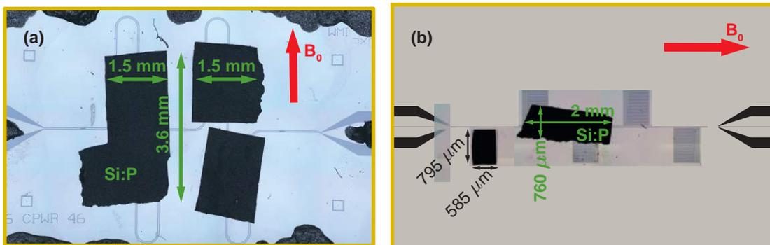
**Figure 2.11:** Micrograph of the (a) CPWR and (b) LER loaded with pieces of phosphorus doped  $^{28}\text{Si}$  crystal. The red arrows indicate the orientation of the external static magnetic field  $B_0$ .
