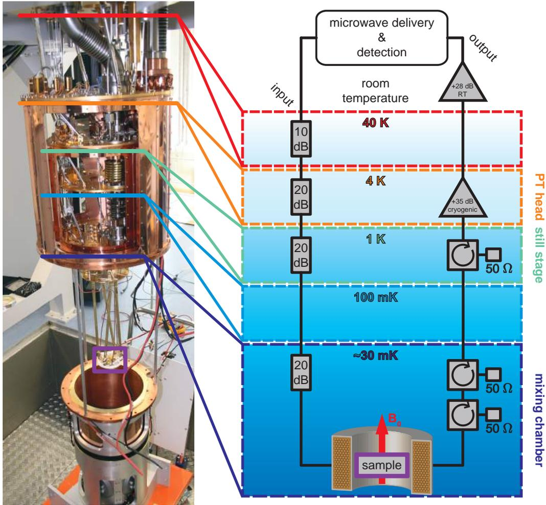
**Figure 2.9:** Image of the open cryogen free dilution refrigerator together with a schematic of its temperature stages, including the microwave circuit and the distribution of its components on the temperature stages. The temperature stages in the image are highlighted and assigned to their corresponding stage in the schematic.
