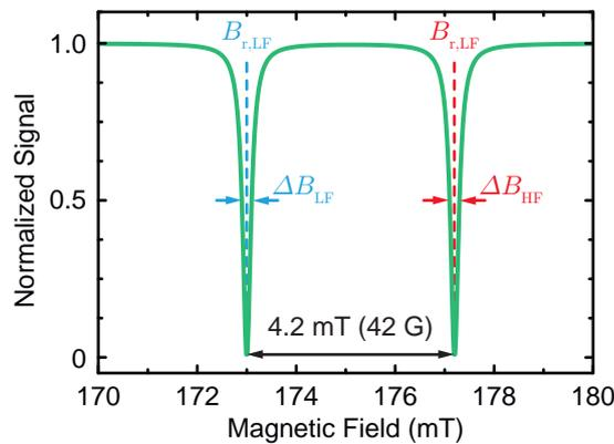
**Figure 2.7:** Exemplary electron spin resonance spectrum (resonance depths and linewidths are arbitrary).
