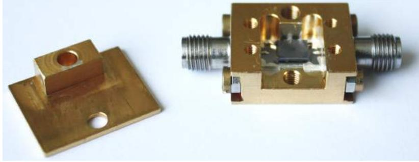
**Figure 2.10:** Photograph of an open gold plated oxygen-free high thermal conductivity copper sample box together with its corresponding lid. The two SMA connectors allow for an easy integration into the cryogenic microwave setup. Mounted into the box is a thin film niobium resonator covered with pieces of phosphorus doped  $^{28}\text{Si}$  crystal. The crystal pieces are held in position by an additional piece of  $^{\text{nat}}\text{Si}$  substrate.
