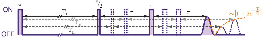
**Figure 4.20:** Schematic inversion recovery pulse sequence, when using the magnitude detection method [125]. Repeatedly applying the sequence, while increasing the wait time  $T$ , results in an echo signal evolution as given in Eq. (4.11). The characteristic time constant of the echo signal evolution corresponds to the longitudinal relaxation time  $T_1$ .
