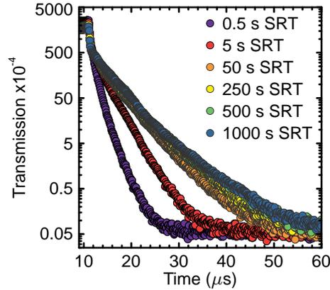
**Figure 4.2:** Logarithmically scaled microwave transmission  $I^2/I_{\text{input}}^2$  as a function of time, showing the falling edge of a  $11 \mu\text{s}$  long pulse with an amplitude of  $2 \text{ nW}$  applied to the CPWR. Each trace is averaged 25 times, using a different SRT (see legend).
