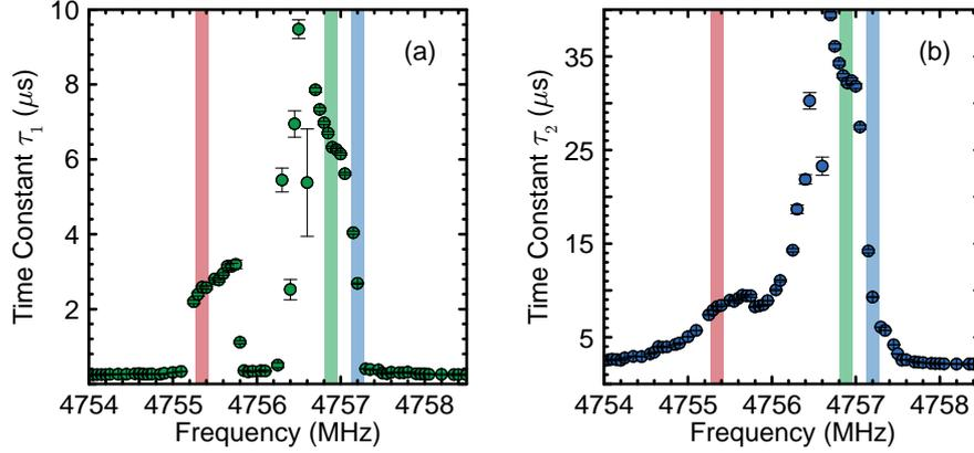
**Figure 4.7:** Time constants  $\tau_1$  (a) and  $\tau_2$  (b) as a function of the pulse frequency, determined by fitting Eq. (4.4) to the spectroscopic data shown in Fig. 4.6 (a). The resonance frequencies of the upper, lower and central hybrid modes are highlighted by blue, red and green bars, respectively.
