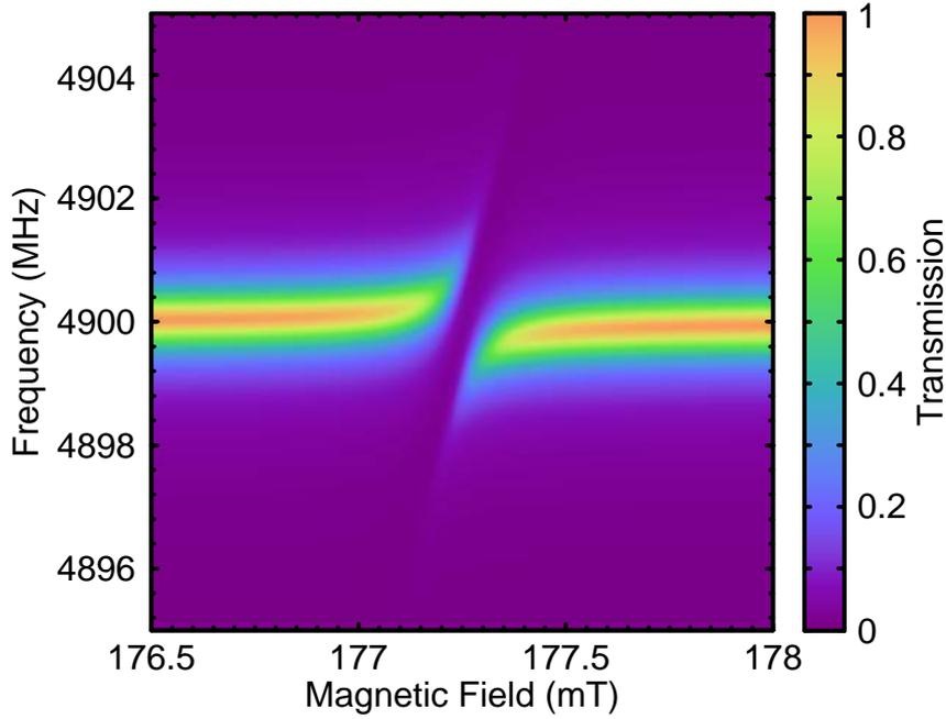
**Figure 3.9:** Color coded normalized power transmission  $|S_{21}|^2$  as a function of frequency and static magnetic field, using  $\omega_r/2\pi = 4.9$  MHz,  $\kappa_0/2\pi = 400$  kHz,  $\gamma/2\pi = 600$  kHz and  $g_{\text{eff}}/2\pi = 1$  MHz. For the spin transition resonance frequency  $\omega_s/2\pi$ , the solution from the spin Hamiltonian (2.10) in Sec. 2.2 for the high field spin transition is chosen.
