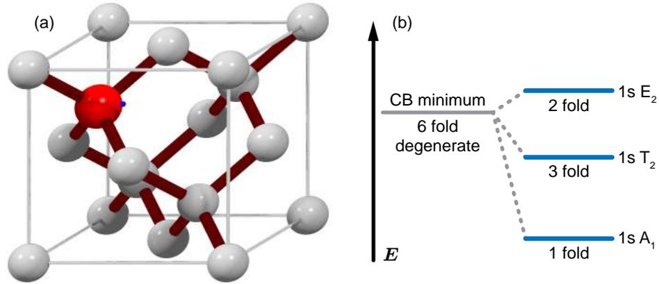
**Figure 2.5:** (a) Schematic of the diamond cubic crystal structure of silicon. The grey atoms represent silicon atoms and the red a phosphorus donor with its accompanying donor electron in blue. The dark red joints between the atoms illustrate their covalent binding, while the outer gray joints serve to define the cubic unit cell. (b) Schematic of the energy levels of phosphorus donors in silicon [59].
