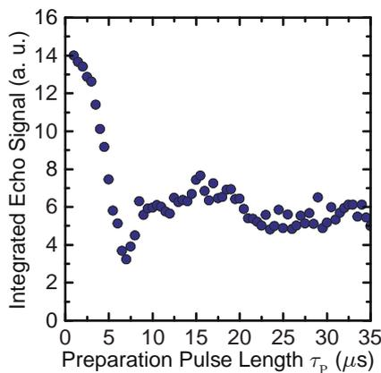
**Figure 4.9:** Echo detected Rabi oscillation, showing the integrated echo signal as a function of the preparation pulse length  $\tau_p$  at 50 mK, using the CPWR. 5 ms after the preparation pulse the echo generation pulse sequence is initiated, consisting of a  $5 \mu\text{s}$  and  $10 \mu\text{s}$  long microwave pulse separated by  $100 \mu\text{s}$  [113].
