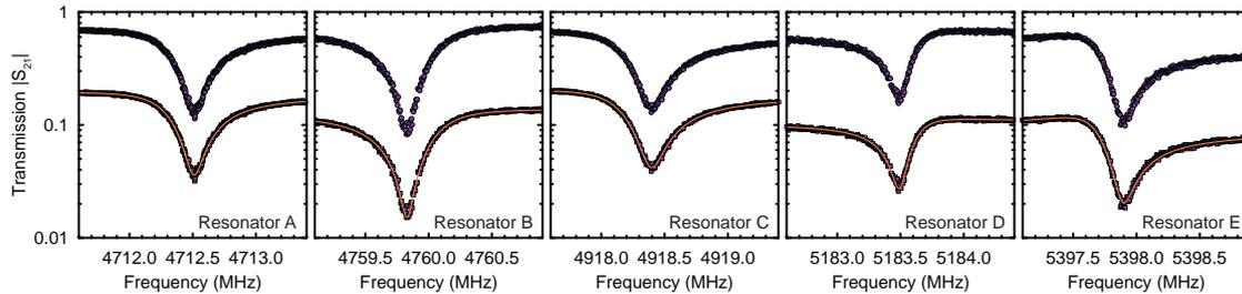
**Figure 3.6:** Uncalibrated (square symbols) and calibrated (round symbols) transmission  $|S_{21}|$  of each LER at 50 mK. The orange solid line represents as fit to the uncalibrated spectra, using Eq. (3.6).
