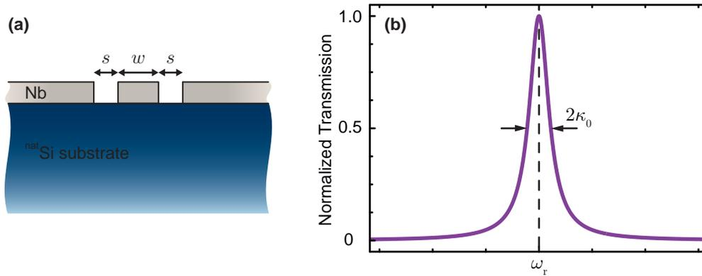
**Figure 2.1:** (a) Schematic of a CPW cross-section including the center conductor width  $w$  and the gap width  $s$ . (b) Exemplary normalized transmission spectrum of a CPWR resonant mode. The transmission peaks at the resonance frequency  $\omega_r$  and exhibits a Lorentzian lineshape with a half width at half maximum  $\kappa_0$ .
