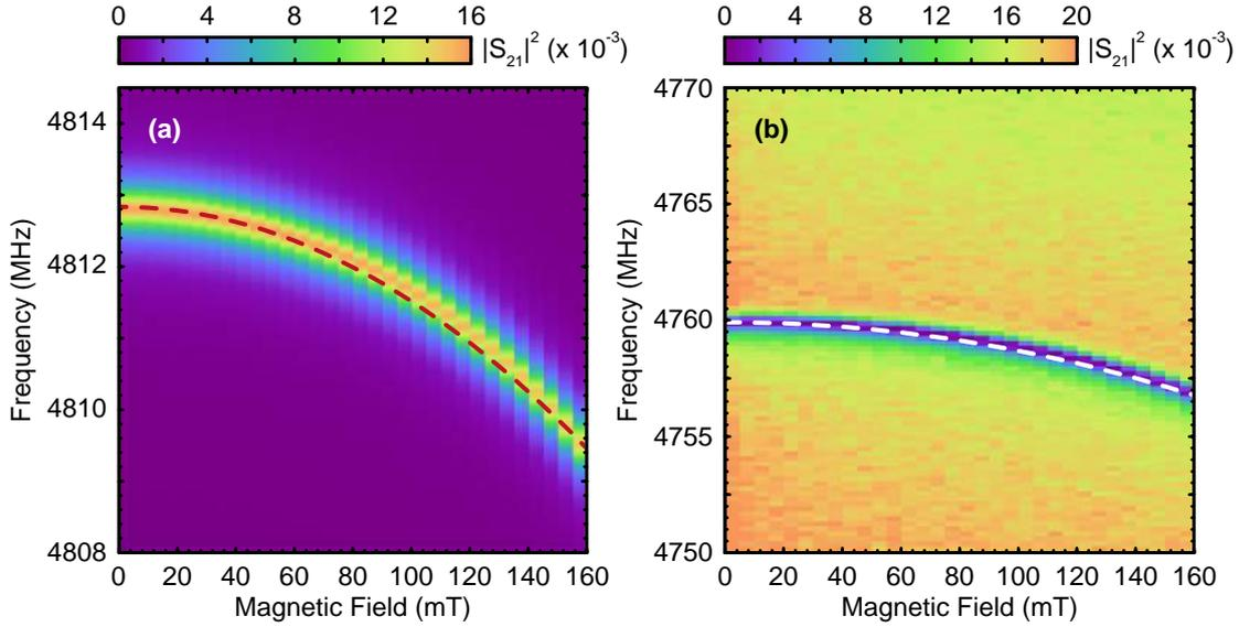
**Figure 3.7:** Uncalibrated power transmission  $|S_{21}|^2$  of a (a) CPWR and (b) LER, as a function of the VNA frequency and static magnetic field  $B_0$ . The dashed lines in the spectroscopy data are fits to the resonance frequency dispersion, using the dependence defined in Eq. (3.9). The CPWR measured in spectrum (a) is made of a 200 nm thick niobium film, instead of a 150 nm thick film, but is otherwise of equal design.
